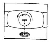
cover and turn the cover counterclockwise to the "open" position. Remove the cover.
